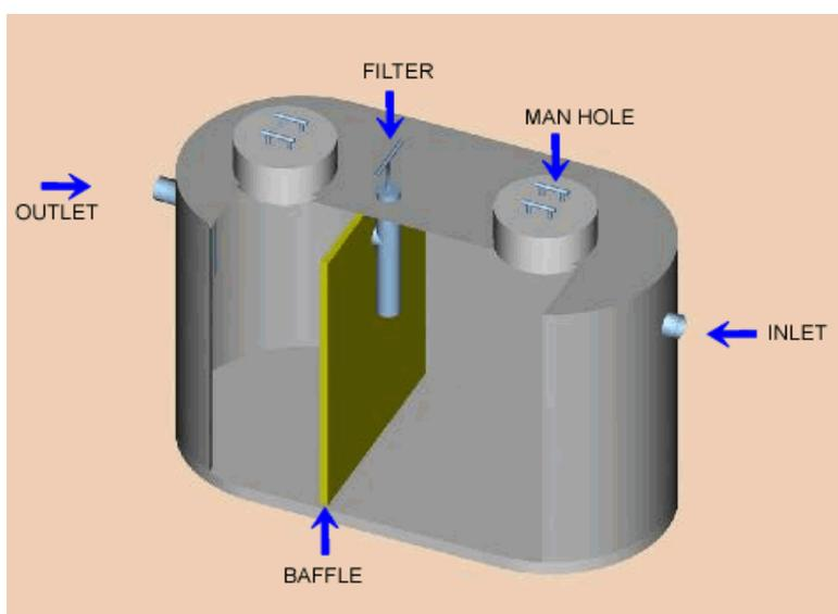
If your system is based on an older style septic tank it may have a separate pump chamber buried next to it, then the filter will be right at the end of the septic tank.
