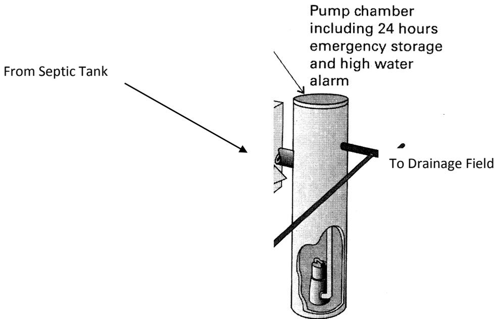
Otherwise the Pump will be under the manhole cover furthest away from the house.
